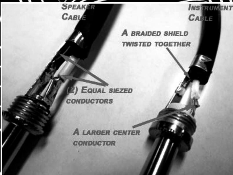
**If you can unscrew either 1/4" jack, inside should either be two identical wires (other than color), which would be a speaker cable, or one insulated wire and a second woven or twisted bare shield going around the insulation of the first insulated wire. That's an instrument cable.**
