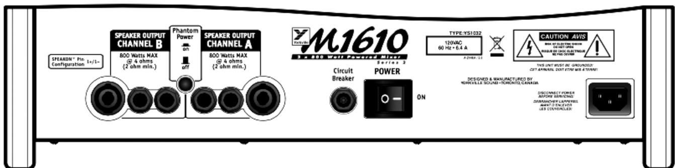
**CABLES:** This is the easy part. These are long cables that have quarter inch plus. The inputs are usually on the back. There is a power supply cable and two cables that go from the speaker output channel jacks at the back of the PA to the jacks in the monitors. Done.
